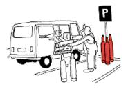
The gas cylinders may remain in the vehicle only in workshop vehicles which are specially designed for that purpose.
