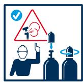
Cylinder valves must be protected against damage by screwing on cylinder caps.
