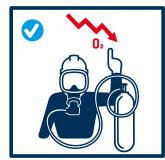
Breathing equipment must be used in situations where oxygen deficiency due to high  $CO_2$  (>3%) content has to be expected.
